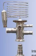
SS Thermostatic expansion valve that modulates refrigerant flow to match system requirements in fluctuating ambient temperatures and compressed air loads. Capillary tube systems used by other manufacturers will increase or decrease refrigerant flow on ambient conditions with no regard to system load. High ambient temperatures or slightly clogged condensers will increase refrigerant flow without a load to balance the system. Operation under these conditions can cause premature compressor failure.
