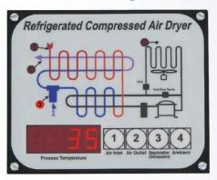
ERF series dryers model are available with an optional digital system monitor. This electronic module monitors air inlet temperature, air outlet temperature, ambient temperature, and separation (dewpoint) temperature. The unit has a 4-20 ma output for data logging or remote system monitoring. The monitor is not a controller and is not integrated into the dryer operation. The monitors independence eliminates the possibility of a dryer shutdown, due to electronic failure.
